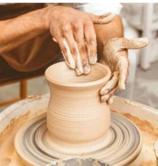
Our patented LEIFELD WSC Flex Technology works flexibly without tools. The principle resembles throwing pottery. The forming movement of the hands is similar to the axial and radial movements of the inner and outer rollers.
